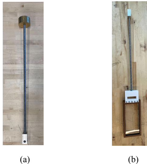
Figure 3: (a) Inertial Tail with coupler (b) Aerodynamic Tail with coupler
